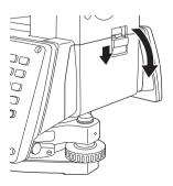
2. Checking the terminal side on the battery, insert the battery as shown.
