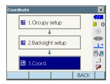
Press [MEAS] to start measurement. Press [STOP] to stop the measurement. The coordinates of the target point are displayed. Select the "Graphic" tab to display coordinates on a graph.
