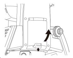
Power OFF the instrument. Connect the USB port
