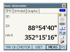
The measured distance data (SD), vertical angle (ZA), and horizontal angle (HA-R) are displayed.
