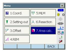
Press [OBS] to display <Area calculation/ measurement>. Sight the first point on the line enclosing the area, and press [MEAS]. Measurement begins and the measured values are displayed. Press [STOP] to stop measuring.
