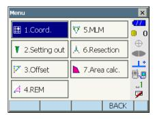
Select "Occupy setup" and enter instrument station coordinates,instrument height (HI) and target height (HR).
