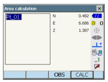
Repeat steps 2 to 3 until all points have been measured. Points on an enclosed area are observed in a clockwise or counterclockwise direction.
