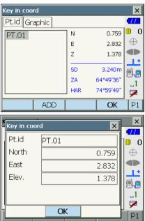
Select a setting-out point in the first screen of step 3 and press [OK] to display <Set out Coords>.  Position the target on the line of sight and press Press [H.TURN] to automatically rotate the instrument until the angle of the setting out point reads 0°.
