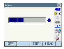
When **[S-LEV]** is pressed, a gauge indicating light intensity is displayed.
