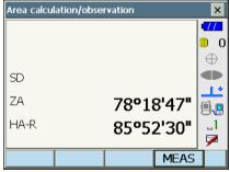
The measurement results are displayed. Press [YES] to confirm. The value of point 1 is set in "Pt 01".
