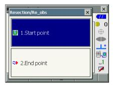
Press [OK] to finish resection measurement and return to <Resection/Menu>. Only Z (elevation) of the instrument station coordinate is set. N and E values are not overwritten.
