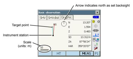
The "Graphic" tab display can be modified using the softkeys in the second page.
