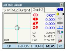
Press {ESC} to return to <Key in coord>. Set the next setting out point to continue setting out measurement.
