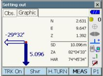
Move the target until the distance to the settingout point reads 0m. When the target is moved within the allowed range, all distance and position arrows are displayed.
