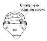
Adjust the adjusting screws until the tightening tension of the three screws is the same to align the bubble in the middle of the circle.
