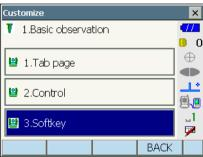
Select the desired tab. All softkeys currently allocated to each page of that tab are displayed.
