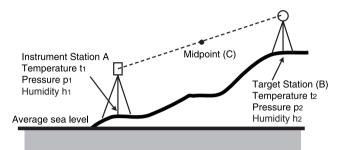
• If the weather correction is not required, set the ppm value to 0.
