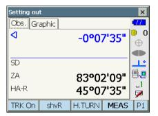
5. Sight the target and press [MEAS]. Measurement begins and the measurement results are displayed.
