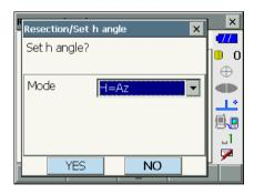
Press [NO] to return to <Resection/Menu> without setting the azimuth angle.
