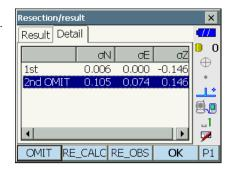
Press [RE CALC] to perform calculation again without the point designated in step 7 The result is displayed.
