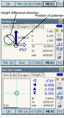
Move the target to find the correct distance (0 is displayed) to the setting out point.
