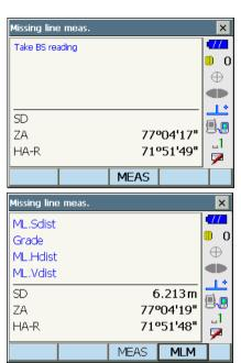
Results for measurement between starting position and second target
