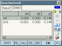
If there are problems with the results of a point, align the cursor with that point and press [OMIT]. "OMIT" is displayed to the right of the point. Repeat for all results that include problems.
