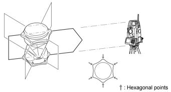
When using the ATP1S, the 360° Prism should be set up so that a pair of diametrically-opposed marks on top of the prism are aligned with the sighting direction of the instrument.
